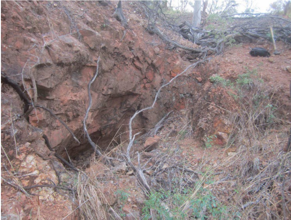
Plate 1: Lady Franklin Workings. Photo of pit showing shallow inclined shaft excavated on the main lode. Some mineralised quartz vein material remains exposed at lower left hand side of photo. View looking west along line of workings.
