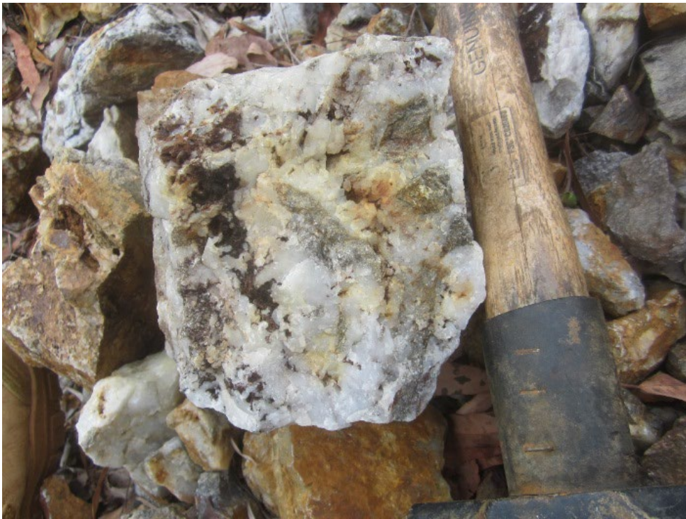
PLATE 3: Lady Franklin ore sample. Brecciated phyllite, white, medium grained, euhedral quartz crystals lining breccia clasts and limonite after sulphides filling matrix cores.
