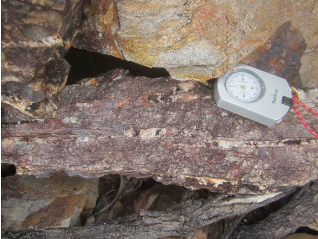
PLATE 7: Mullock from All Nations main pit showing quartz – limonite (after sulphide) vein sets hosted in greisen (coarse quartz – mica alteration).
