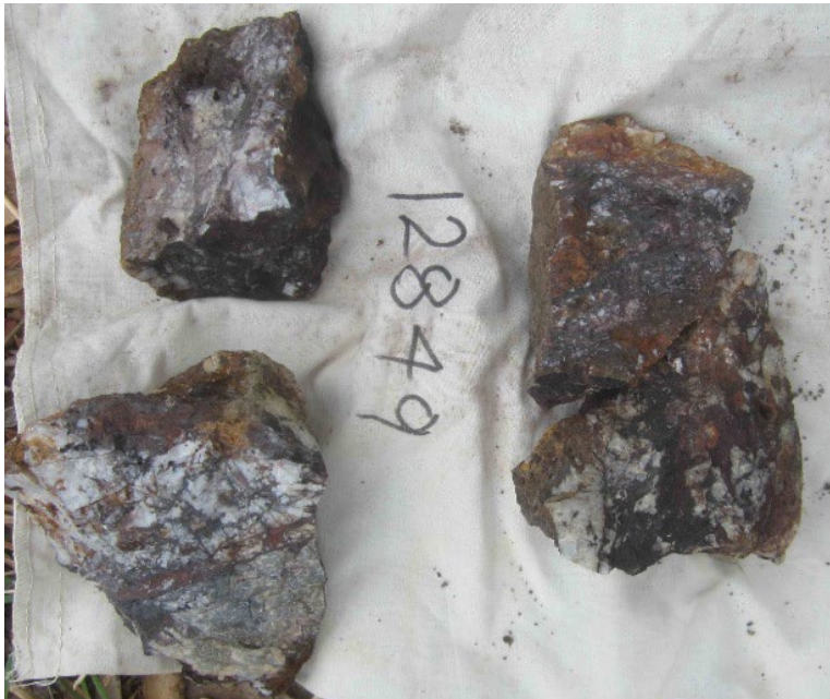
PLATE 5: Sample of ore from the Canadian reef. Shows white to grey, fractured and recrystallised quartz cemented by limonite after sulphides (sample # 12849, 3.70 g/t gold).
